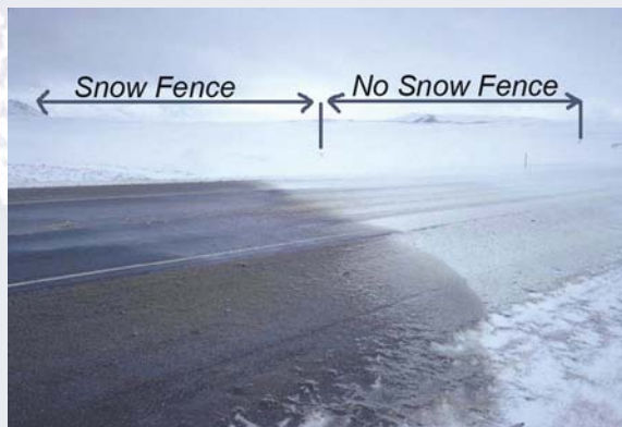
Figure 1. Transition from frozen slush to wet pavement corresponds to the beginning of the area protected by a 12.4-ft snow fence located about 500 ft upwind.
