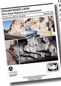
p-236 Ground-Based **LIDAR Rock Slope** Mapping and **Assessment (FHWA** September 2008) LiDAR (Light Detection and Ranging), also referred to as 3D laser Scanning, is an emerging threedimensional mapping technology that employs a laser and a rotating mirror or housing to rapidly scan and image volumes and surficial areas such as rock slopes and outcrops, buildings, bridges, and other natural or
