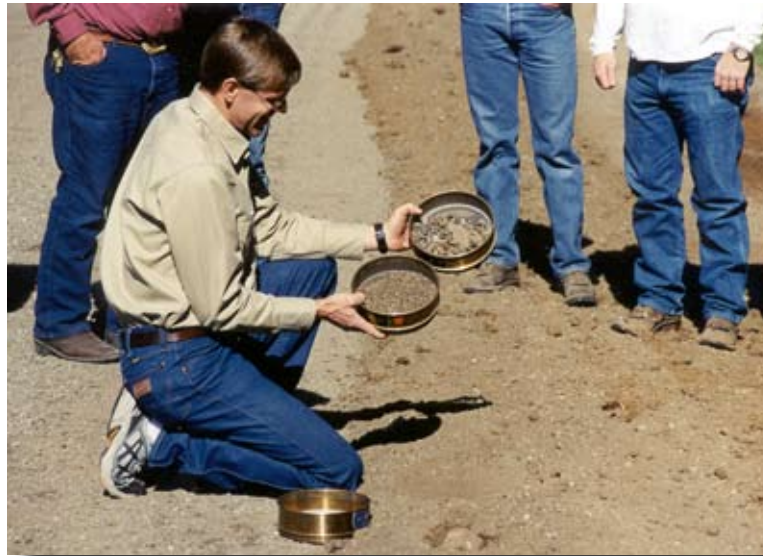
Montana LTAP Director Steve Jenkins demonstrating the use of sieves to determine soil types.
