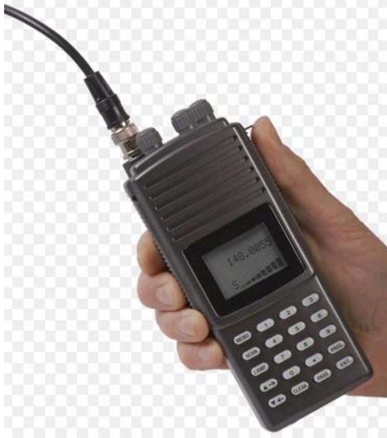
Figure 5.6: The Communications Specialists R-1000 Telemetry receiver. Gathered from the Communications Specialists website.
