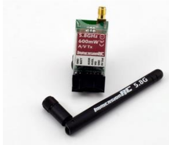
Figure 5.3: The ImmersionRC 600mW 5.8GHz A/V transmitter. Gathered from the ImmersionRC website
