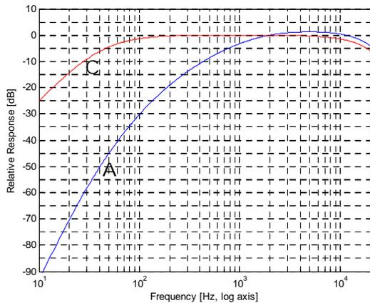
Figure 2: A-weighting and C-weighting filters
