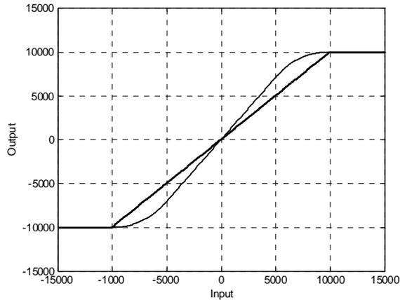
Figure 1: Hard clipping function (straight segments) and soft clipping function (curved segment)
