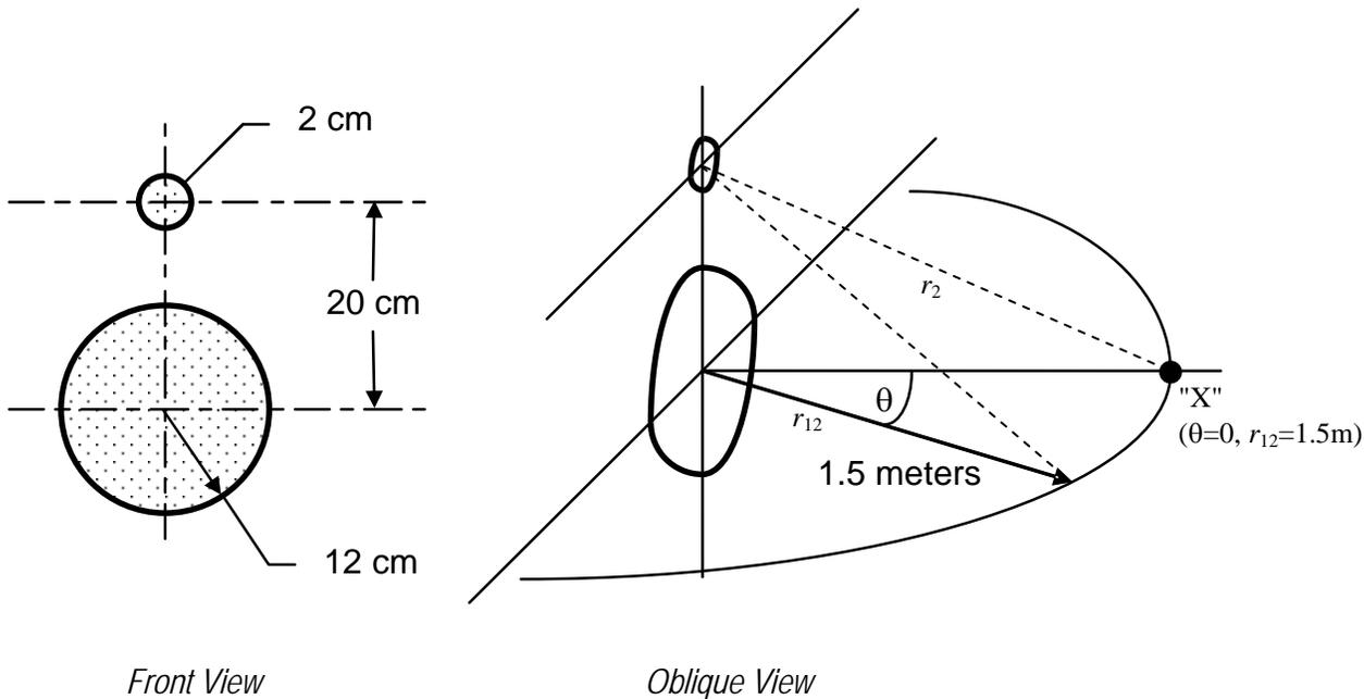
Each driver is modeled as a baffled piston radiator (far field case, K&F §7.4b, pp. 181-184). Both drivers are operated at  $f = 5 \text{ kHz}$  into air at  $20^\circ\text{C}$ .
