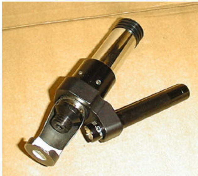
Figure 20. Scaled Loupe Used to Monitor Crack Fronts
