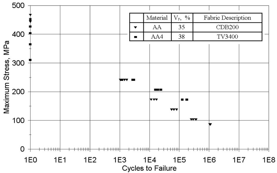
Figure 3. Comparison of Tensile Fatigue Data For Triax Fabric Laminates, R = 0.1
